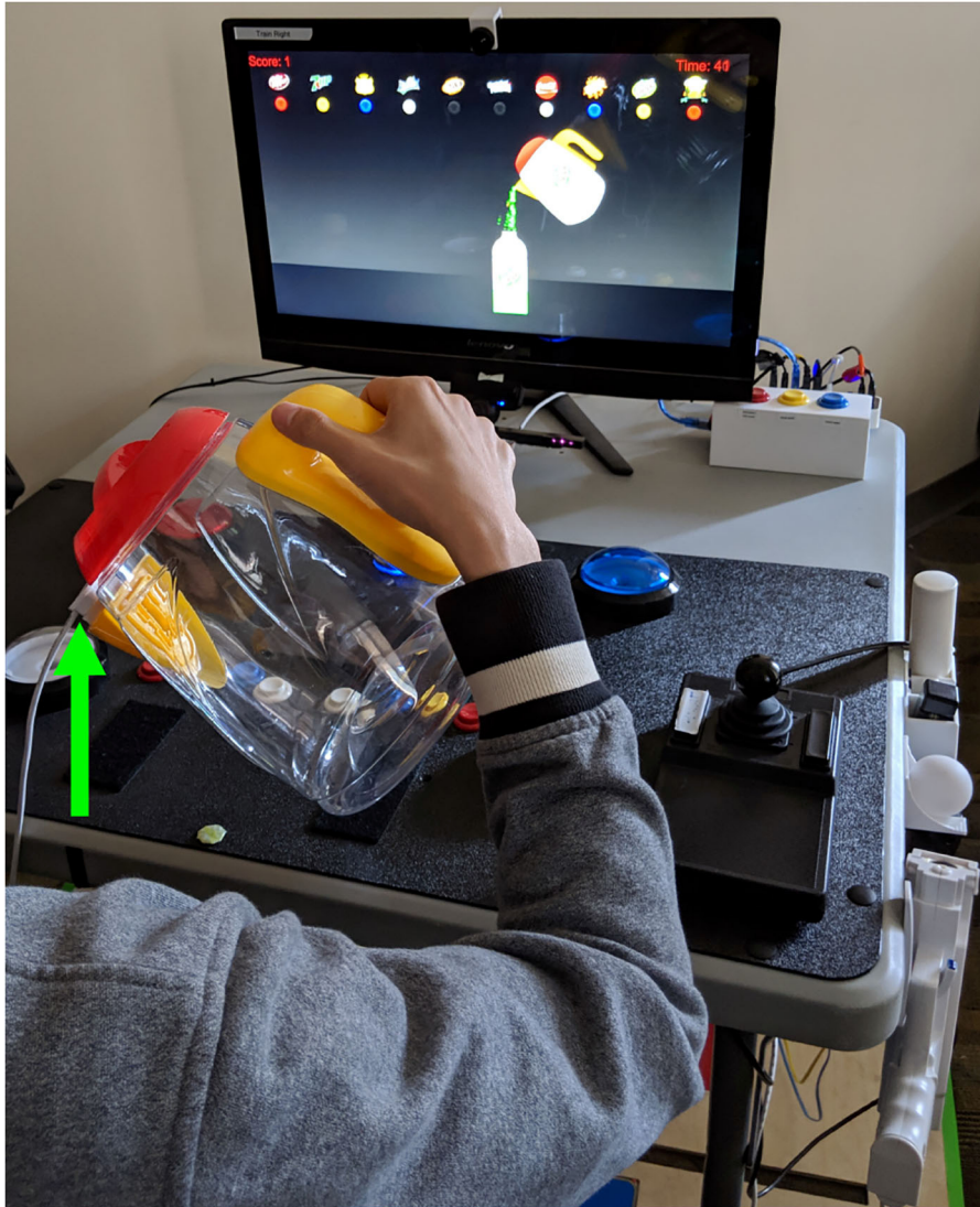
FIGURE 3 | Sensors were attached to real objects to play a game that drives an iADL. The patient grasped an actual water pitcher onto which an accelerometer (green arrow) was attached magnetically. Accelerometer data were sent to the computer running the TR program. As the subject rotated the hand-held pitcher, the figure of a pitcher on the video screen moved synchronously. In this way, the subject used a real object to play a game, displayed on the TR computer screen, where the goal was to fill empty cups to the correct level.
