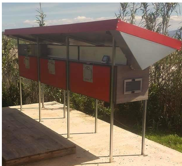
Figure 3.3. Solar dryer used in the shade-drying method. SeaExpert 2020.
