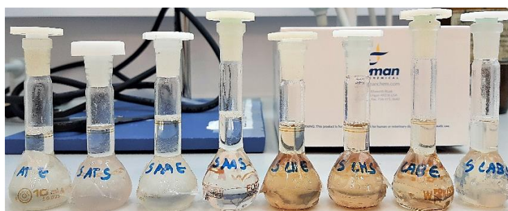
Figure 3.17. Final solutions of 1 mg/mL prepared from the supernatant collected from the aqueous extracts. From left to right: Shade-dried Asparagopsis taxiformis ; Sun-dried Asparagopsis taxiformis ; Shade-dried Asparagopsis armata ; Sun-dried Asparagopsis armata ; Shade-dried Cystoseira humilis ; Sun-dried Cystoseira humilis ; Shade-dried Cystoseira abies-marina ; Sun-dried Cystoseira abies-marina . Diana Julião, June 2020.
