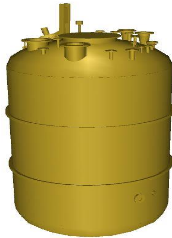
Figure 2. Batch reactor to produce various resins in Hexion Kitee.
