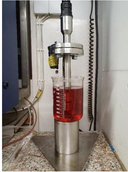
Figure 14. NIR probe is put to analyze the hazardous samples in manufacturing laboratory of the Kitee plant in 2020.
