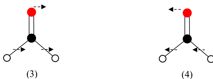
Figure 5. The illustrative demonstration of the symmetrical and the asymmetrical bending vibrations. (Retelld Workman & Weyer 2008, p. 6)
