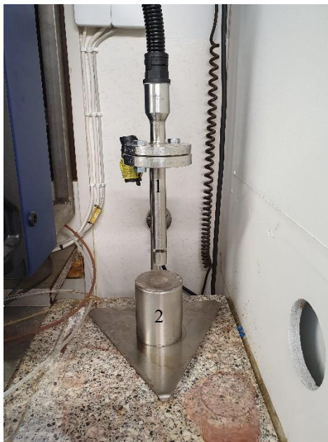
Figure 13. NIR probe to measure the hazardous samples in the manufacturing laboratory.
