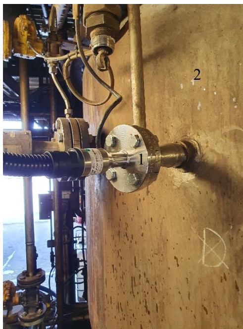
Figure 12. NIR probe (1) have installed in the side of the batch reactor R204 (2) in the manufacturing area.
