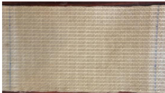
Figure 5: Geotextile specimens after laboratory mechanical damage.
