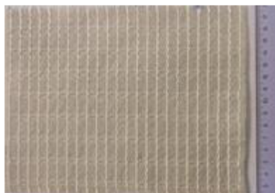
Figure 1: Photograph of the high-strength geotextile (ruler in centimeters).
