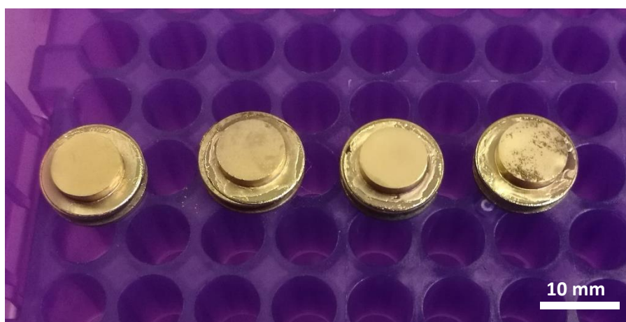
Figure 3.10 – Titanium samples sputter-coated with gold.
