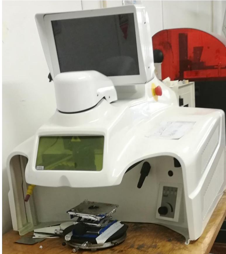
Figure 3.9 – Nd:YAG laser 2 (LM-D 60 7500W, SISMA, Italy)
