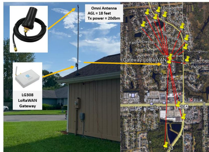
Figure 4.22: The LoRa Testbed Showing Gateway (left) and FTD (right) using the “Google Earth”
