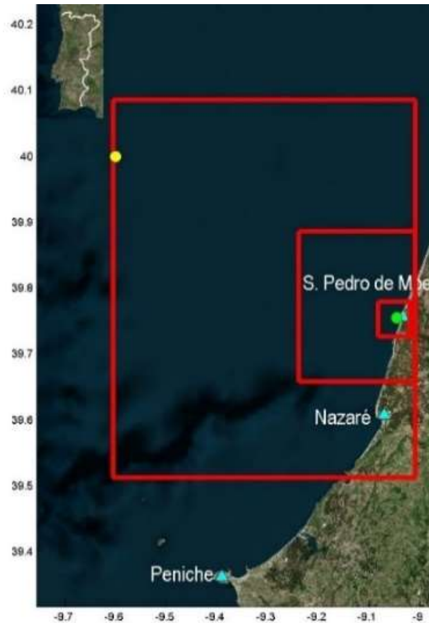
Figure 4.4 - Map with the computational grids using in SWAN. The larger is the main grid and the other two are the nested grid. The yellow point corresponds to the wave conditions input, and the green point corresponds to the location of the wave conditions output (Figure made using MIRONE (Luis, 2007)).
