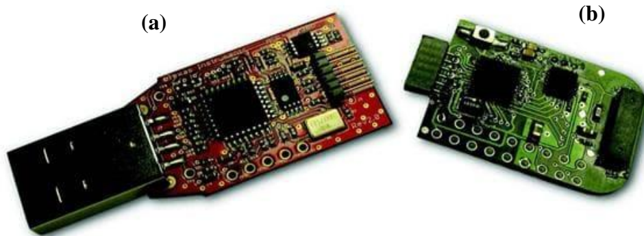
Figure 4.4 - eZ430-TMS37157 tag (b) with the debugger (a). Adapted from [54].
