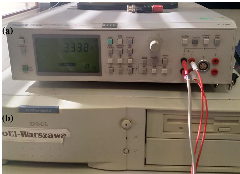
Figure 3.10 - a) Fluke PM6306 LCR meter with b) computer
