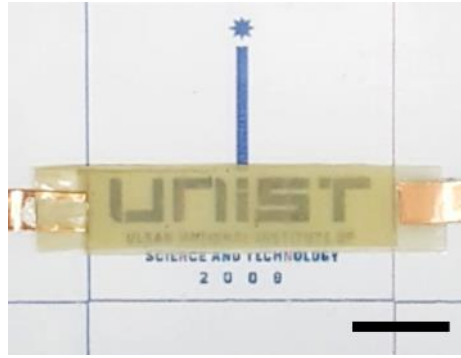
Figure 6.4 Photograph of the fabricated stretchable EL loudspeaker device placed on the background UNIST logo. The scale bar is 1.5 cm.
