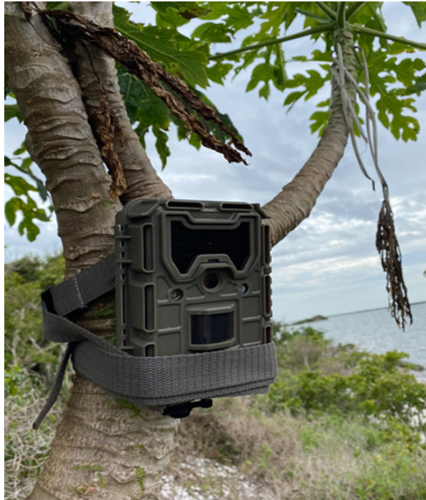
Figure 2. Bushnell “Trophy Cam HD” attached to a tree within the surrounding vegetation on the living shoreline site.
