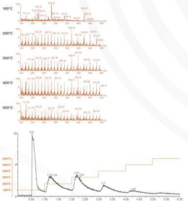
A thermal desorption temperature profile from a lubricant oil sample acquired using a temperature ramp method from 100 °C to 600 °C. Various lubricant oil additives, including Irganox 5057 and Antioxidant L57, were detected at low temperature. Different components of the lubricant oil and other high boiling additives started to desorb at 200 °C and were observed up to 500 °C.
