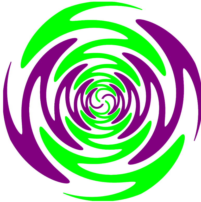
Figure 4.7: The sinuous antenna design has two distinct arms for polarisation separation [16] . The design of the antenna allows for a relatively small cross-section for the bandwidth it is designed to respond to. It is also a planar antenna allowing for it to be printed directly on to a PCB while minimising antenna cross-talk when incorporated as part of an array. The orthogonal arms of the antenna allow to differentiate between orthogonal polarised light. Figure taken from “Dual-polarisation broadband sinuous antenna and microstrip power divider design for the Synthetic Aperture Microwave Imager-2 diagnostic” [15]
