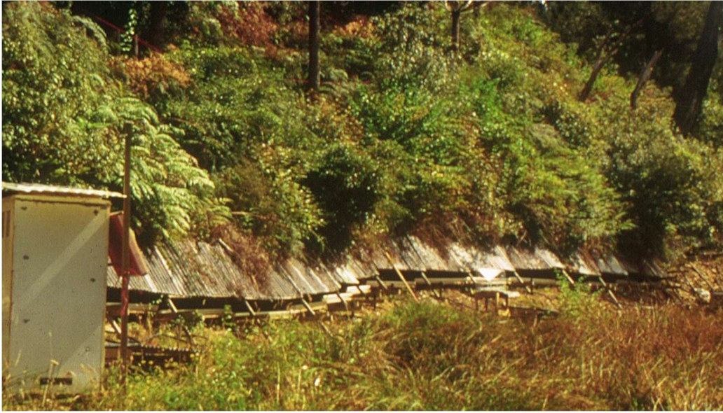
Figure 4. The Woods & Rowe (1996) trench with 30 troughs of 1.7 m length in two groups across the 60 m slope portion. Tipping buckets recorded flow. Subsequent studies on this slope section performed isotope tracing, line source breakthrough experiments and forensic analyses of the soil and bedrock surface above the trench. Photo credit unknown.
