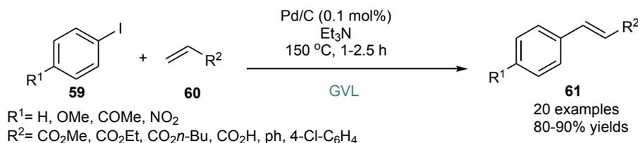
Scheme 26. Mizoroki-Heck reaction catalysed by Pd/C in GVL.
