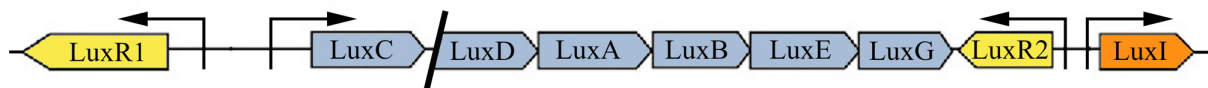
Figure 4 The schematic arrangement of the lux operon and the luxR1/luxR2 genes in A. salmonicida LF11238.
