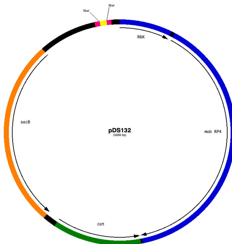
Figure 15: Plasmid map of pDS132 (5286 bp). Properties and restriction sites used in this project are indicated.
