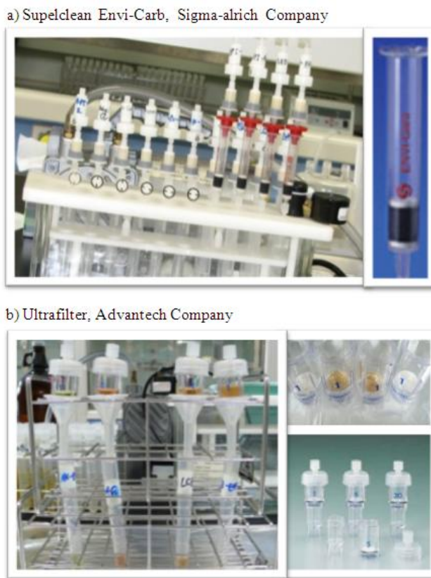
Figure 5.12 Matrix removal procedures a) Supelclean Envi-Carb b) Ultrafilter
