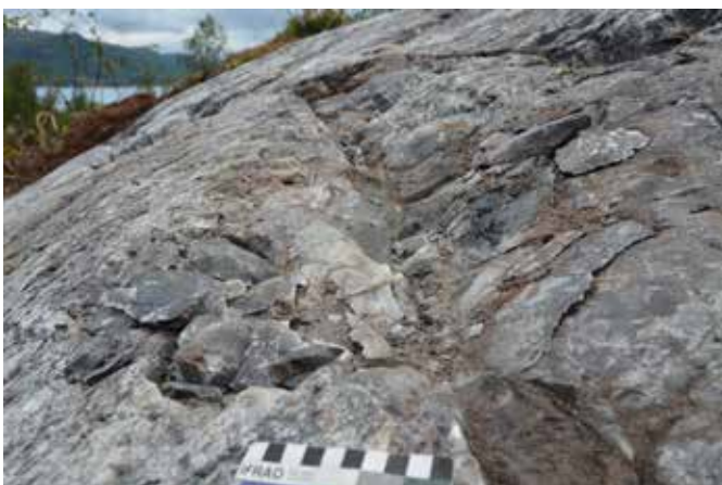
Figur 155 Crack pattern from a single fire (LAB1) burnt for about half an hour, after careful removal of remaining wood and charcoal.
