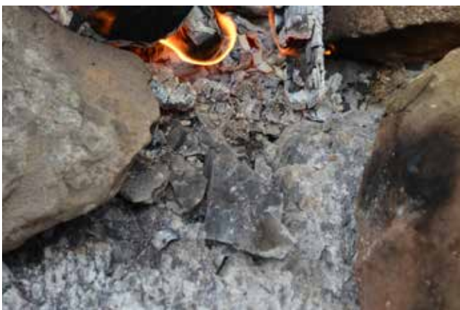
Figur 153 Early cracking of chert into small pieces unusable for tool production, after some 10-15 minutes, LAB1. Note that the chert has not become milky white, implying that the temperature will have been c. 3-400°C
