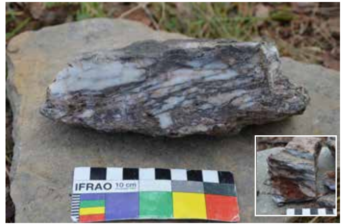
Figur 147 Chert piece (B1, before, left, and after burning) with layers of schist (rich in mica). It burnt in the middle of the fire for a couple of hours (presumably by c. 500°C). The piece was totally cracked along the schist afterwards and the chert got milky white. The schist layers became earthy and red-coloured.
