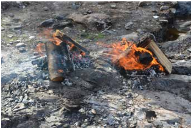
Figur 157 Two fires in LAB2 created deeper cracks between the fires, to some extent following cleavage (arrow).
