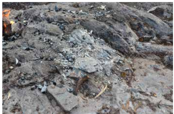
Figur 156 Crack pattern from a single fire (LAB2) burnt for about half an hour. Removal of charcoal has not taken place. Potlid flakes and convex forms on the bedrock could be observed on removal)
