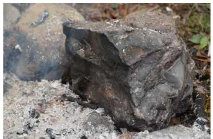
Figur 149 Chert piece (B3, before, left, and after burning). The piece is in brecciated bluish chert with fragments of greyish material. It stood at the perimeter of the fire for 5-6 hours and would have experienced temperatures slightly above 300°C. This temperature was not high enough to create cracks or to make the chert milky white, but some parts with mica became slightly reddish. Moreover, a few flakes peeled off the side oriented toward the fire
