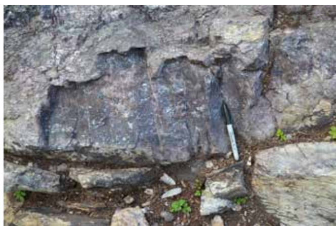
Figur 143 Probable impact of recent frost action in the Melsvik quarry, affecting very poor chert with lots of fissures.
