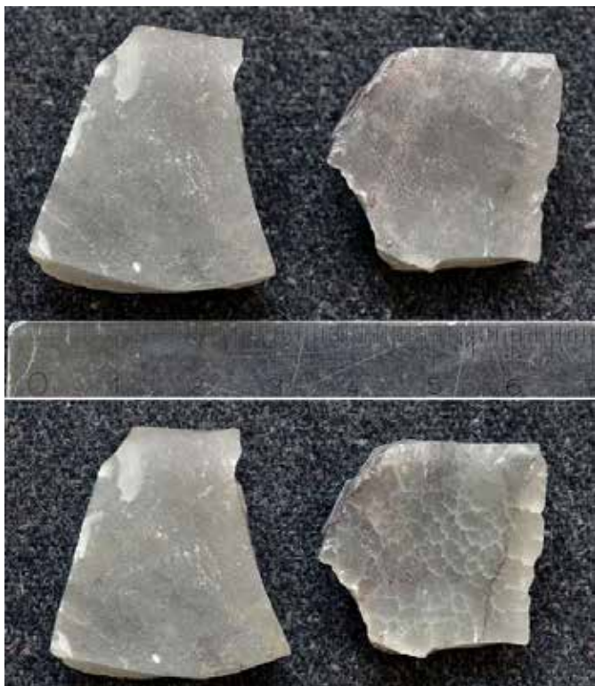
Figur 150 Heating experiment in a baking oven. Top: Two pieces of Melsvik chert before heating. Bottom: The same pieces after heating to 275°C. The left piece was cooled in air, the right piece shock-cooled in water. As can be seen it developed an intensive polygonal crack pattern
