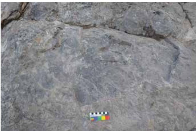
Figur 165 The final forms in the bedrock at LAB5 after fire-setting and cleaning. Note the more jagged forms
