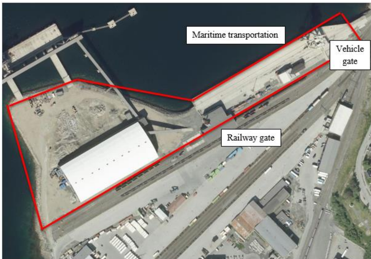
Figure 13 – Illustration of the outline of the suggested passive RFID system.
