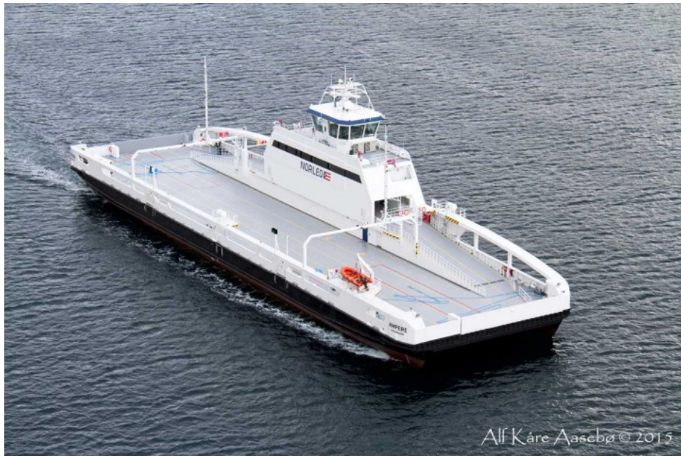
Figure 4.4: Aerial view of the fully electric car and passenger ferry MF Ampere [Stuads, 2015].
