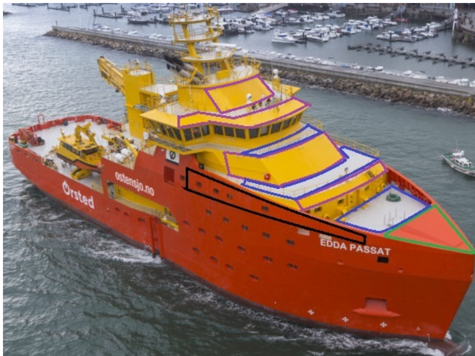
Figure 4.2: Sketch of possible installation areas on Edda Passat. Black area corresponds to \beta = 80^\circ , blue represents horizontal surface, green area corresponds to \beta = 15^\circ and purple represents area with \beta = 35^\circ .
