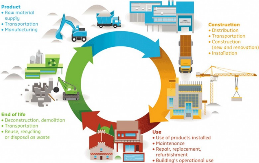
Figure 7: The LCA of a construction product [27]
