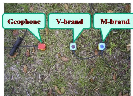
Figure 3. Sensors used for the experiment. Left: conventional geophone. Middle: V-brand MEMS accelerometer. Right: M-brand MEMS accelerometer.
