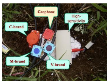
Figure 6. Five sensors fixed to the ground with plaster.
