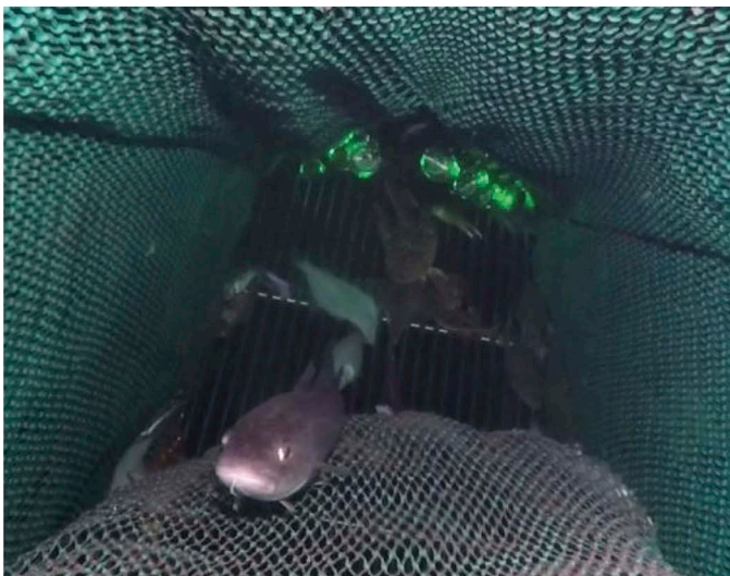
FIGURE 4. Underwater photo from inside the grid section as used during the selectivity experiments with five green Lindgren-Pitman Electralume LED lamps mounted around the escape outlet.
