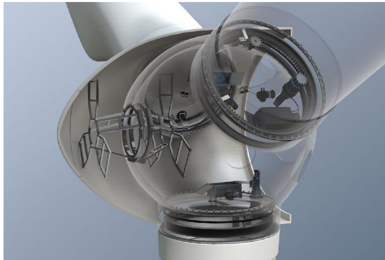
Figure 2-2 HAWT Rotor hub pitch drive. (ifm, u.d.)
