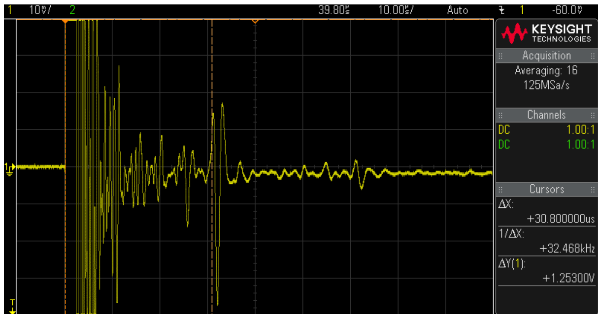
Figure 4-4 Echo response from ultrasonic pulse in simulated crack, second backwall echo
