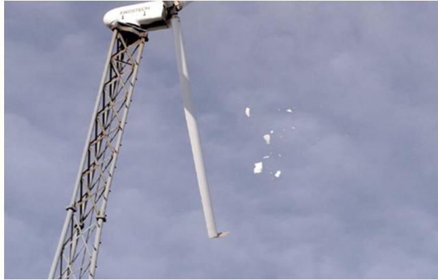
Figure 2-16 Flying ice due to atmospheric icing on rotor blade (Dongsheng, et al., 2015)
