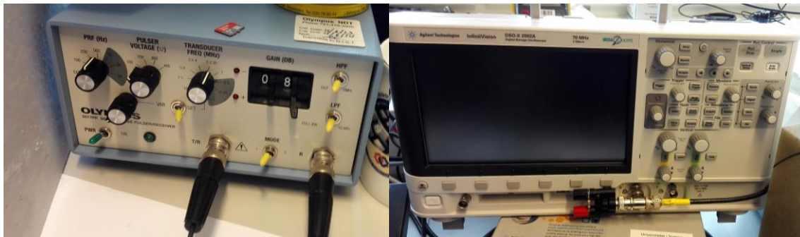
Figure 3-1 Ultrasonic pulser/receiver (left) and oscilloscope (right)
