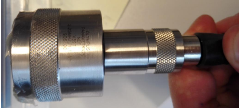
Figure 3-2 V397-SU 29mm element transducer (Skaga, 2017)
