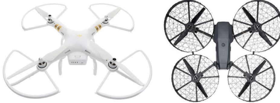
Figure 5-1 Example of UAV propeller guard (left) (DJI Store, 2017) and UAV propeller cage (right) (UAV Expert News, 2017)
