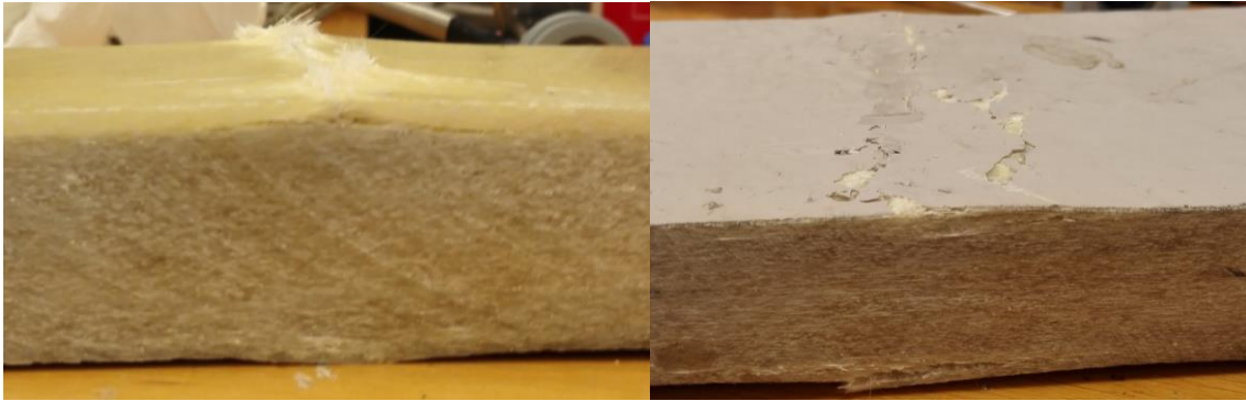
Figure 4-6 Image of visual damage induced in 29mm glass fibre sample by 3-point bending test. Uncoated surface (left) and coated surface (right)
