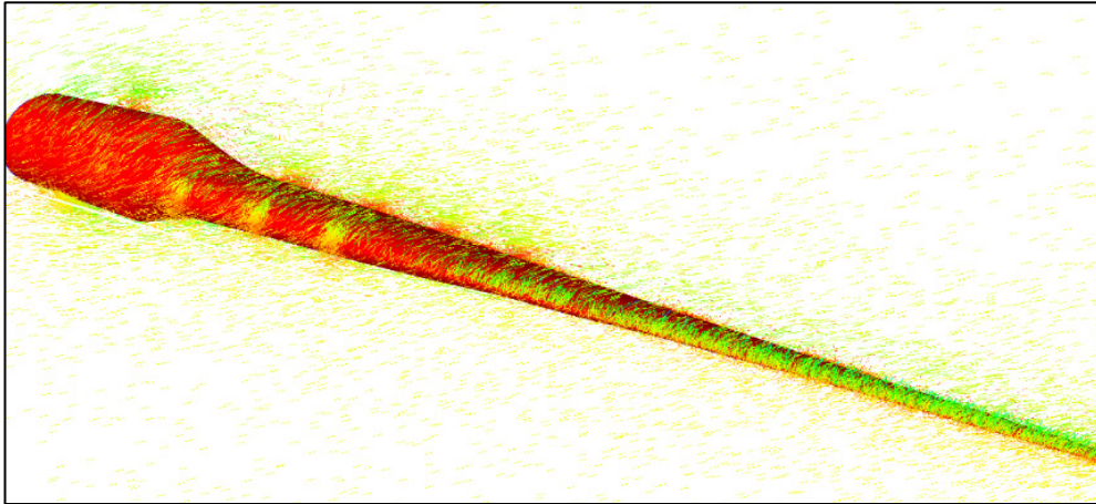
Figure 3: Free stream velocity vectors across wind turbine blade at v=10 m/sec
