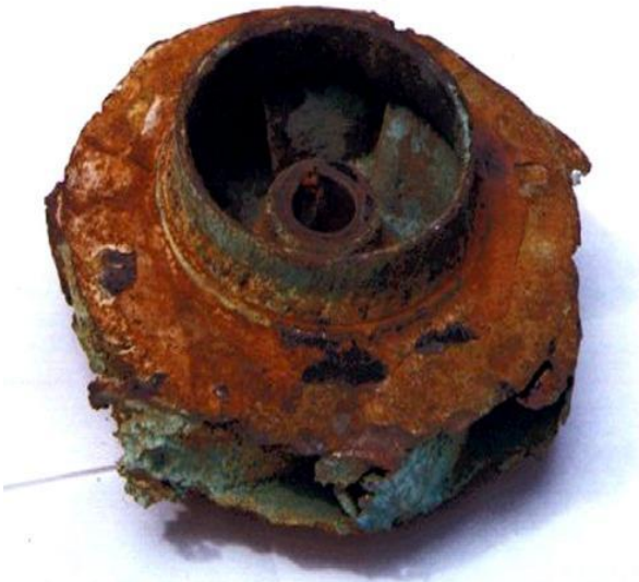
Corrosion & erosion © Simsite
