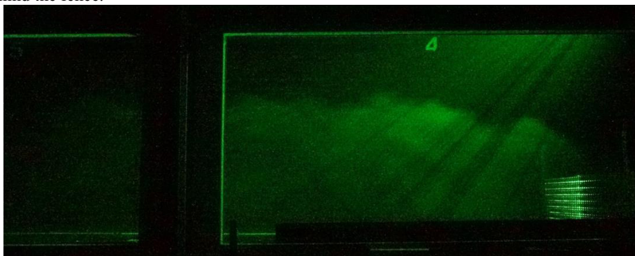
Fig. 4: Visualization of the fence with 23% porosity
