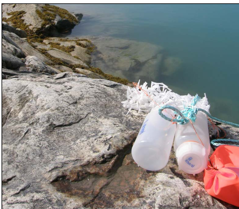
Figure 5. POM together with floating and marking devices, ready to be deployed for three months in the inner parts of Godthåbsfjord.
