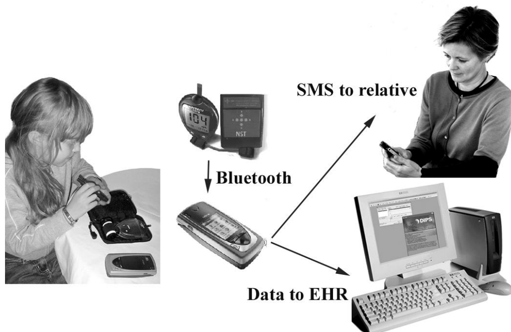
Fig. 20. Overall architecture of the no-touch wireless system for blood glucose transfer (Adapted from Paper 3 [384], Fig. 2).
