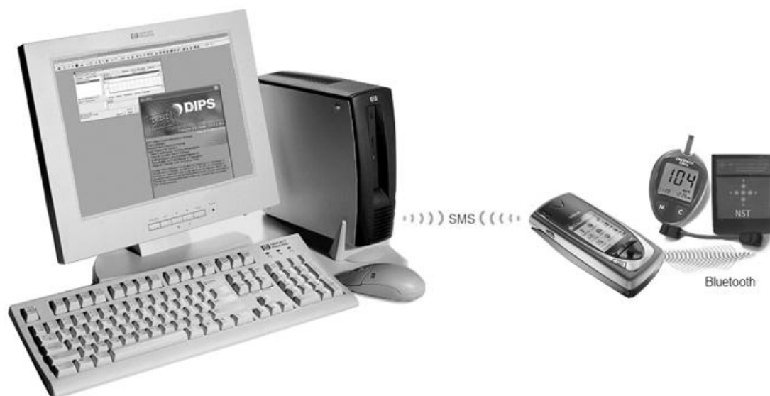
Figure 1 – Transfer of blood glucose measurements into the DIPS EHR system
