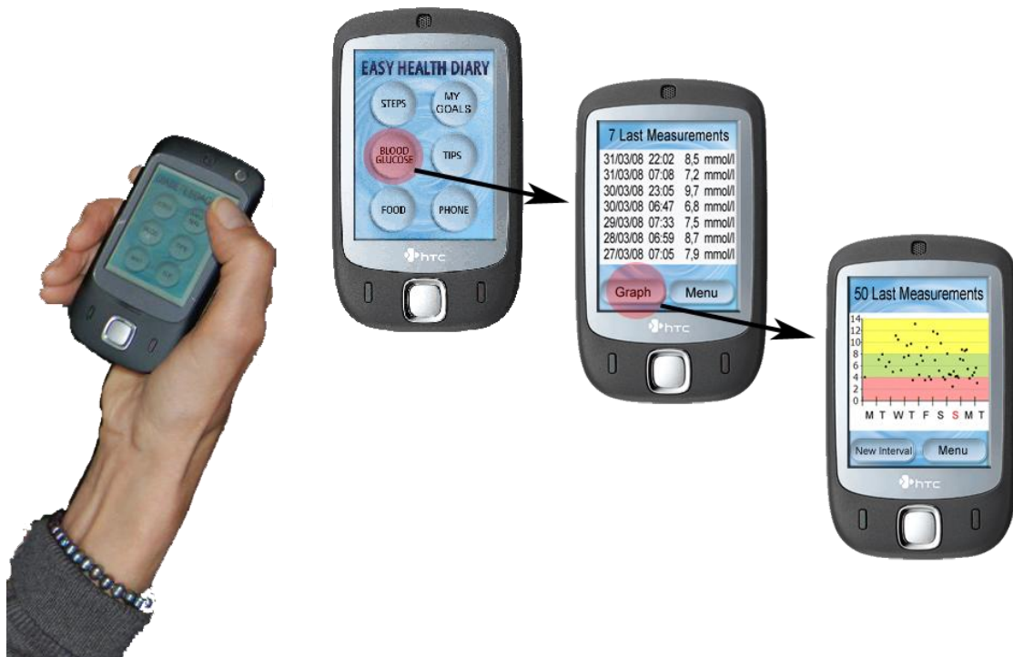
Fig. 21 The blood glucose module of the Few Touch application; the red circle indicates choices made and arrows point to subsequent screen feedback.
