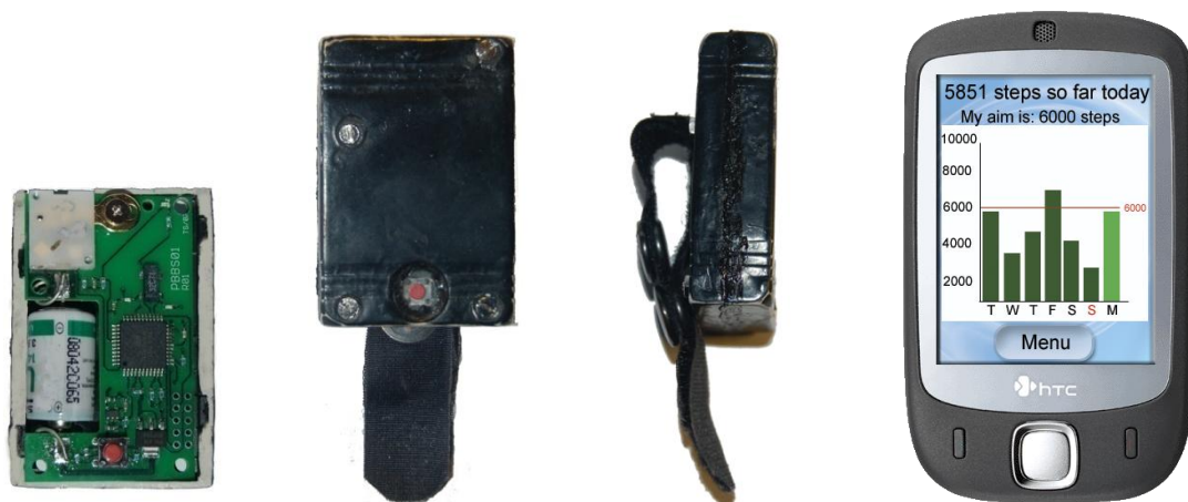
Fig. 23 The final prototype; the electronics, front view, side view, and the feedback screen on the mobile phone.
