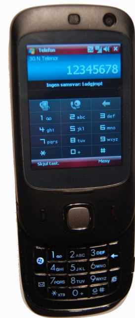
Fig. 11. The HTC “Touch Dual”, with both touchscreen and physical key interface.
