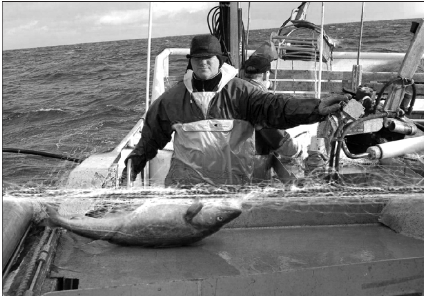
Figure 4. Onboard a modern Norwegian small-scale fish capture machine with fish, people gear and all its devices. The skipper is steering with his right hand, and is controlling the hydraulic hauler with his left hand, while the net clearing device is hanging at the stern. (Photo: J.P. Johnsen)
