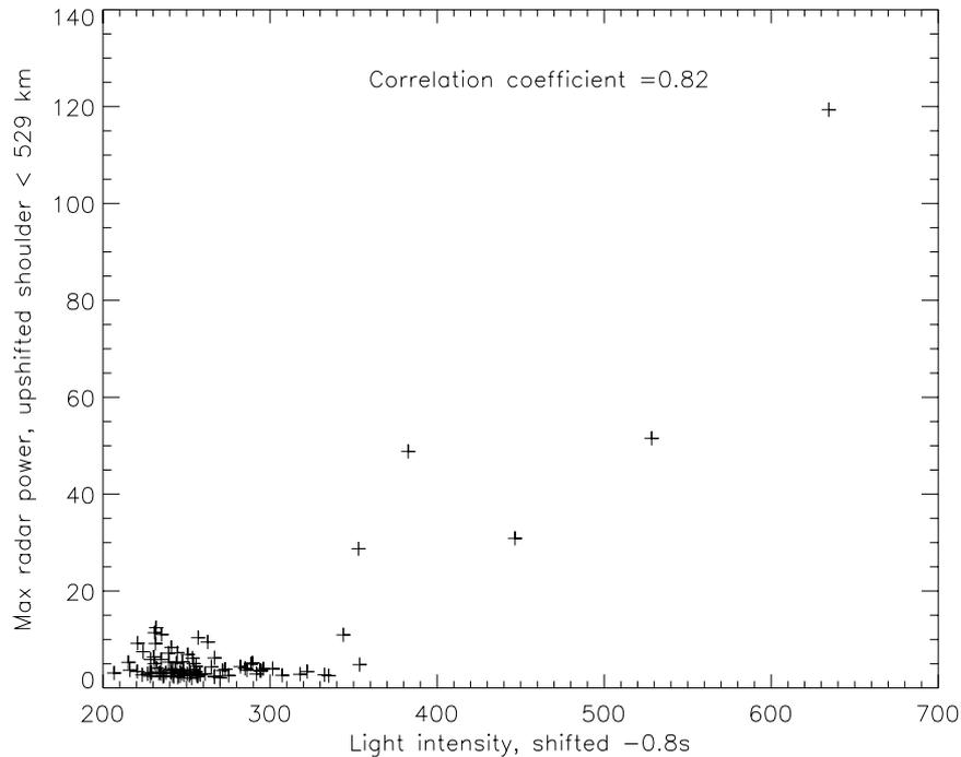
**Fig. 15.** Scatter plot of normalised light intensity (arbitrary units) versus maximum power (arbitrary units) in the upshifted shoulder of the received radar spectrum (taken below 529 km). The light intensity stems from the time series taken from region b1 in Fig. 5, delayed by 0.8 s.
