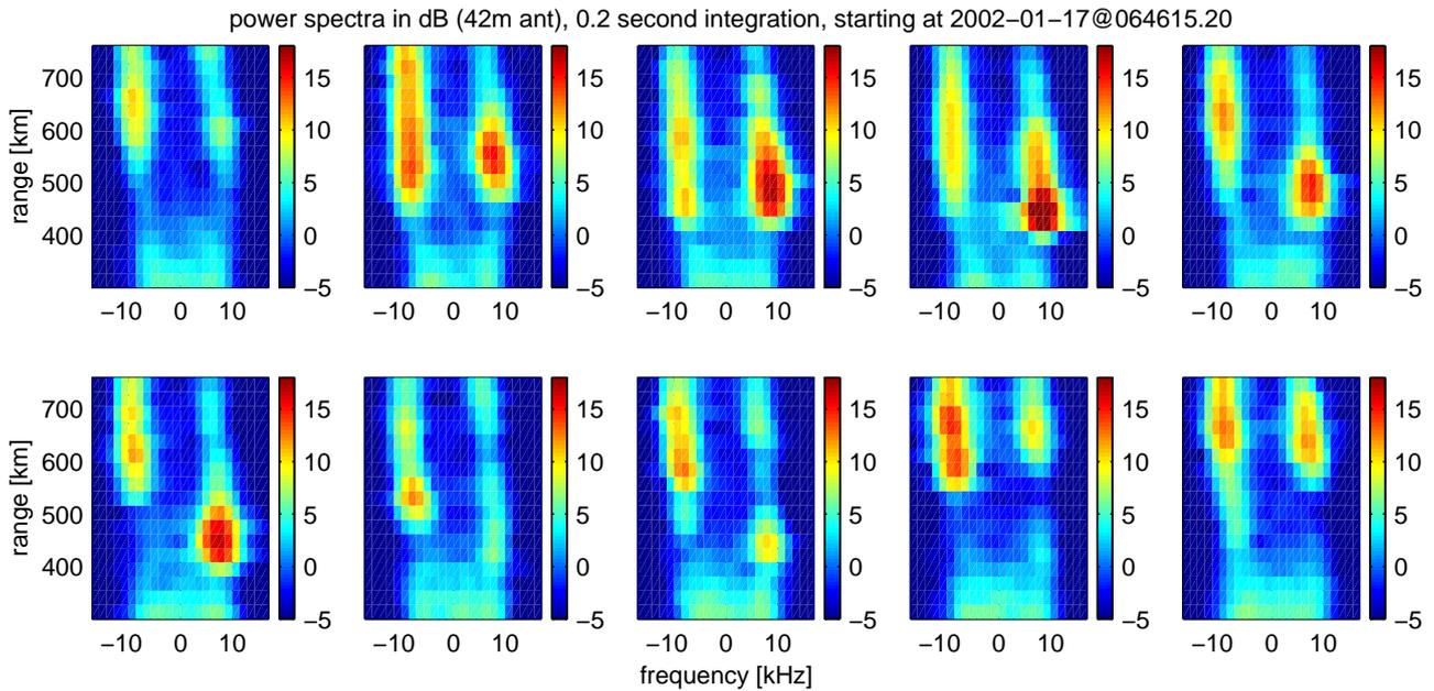
**Fig. 9.** Example of how an event develops in time. Each panel shows powerspectra from the 42 m antenna, in dB, on the same scale for successive 0.2 s integration periods, 2 seconds total. The background noise has not been subtracted, and range<sup>2</sup> attenuation has not been corrected for. We see for example how one range-frequency region (+10 kHz at 450 km) shows an increase in scattering by 15 dB in 0.6 seconds, and then fades back to its original value within the next second or so.
