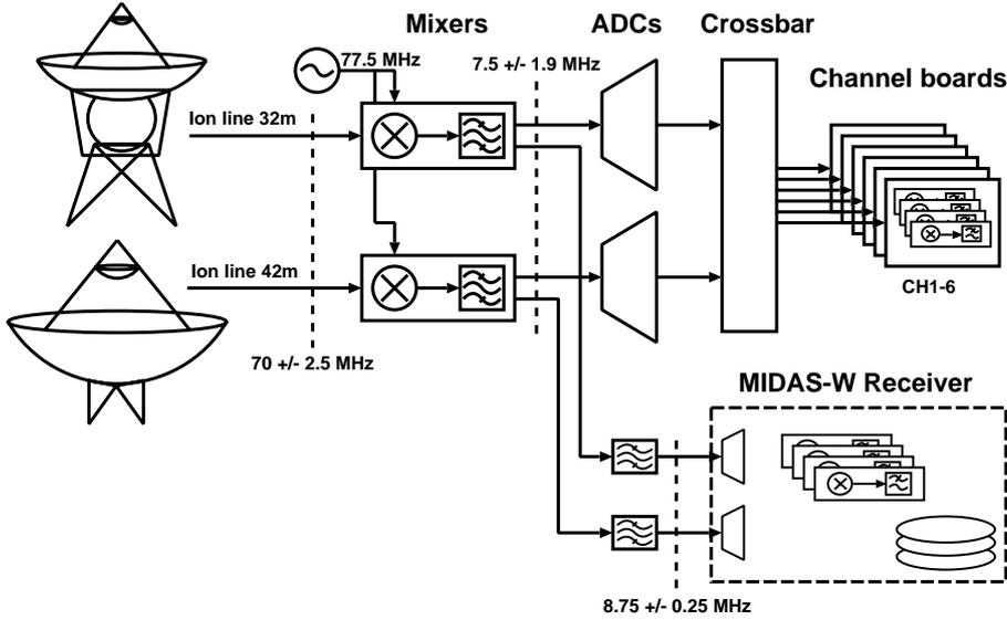
**Fig. 1.** Block diagram of the ESR analog/digital receiver showing the path of the signal through the system and how the MIDAS-W receiver is connected to the existing system. The vertical dashed lines at various points show the center frequency and bandwidth of the signal at those stages
