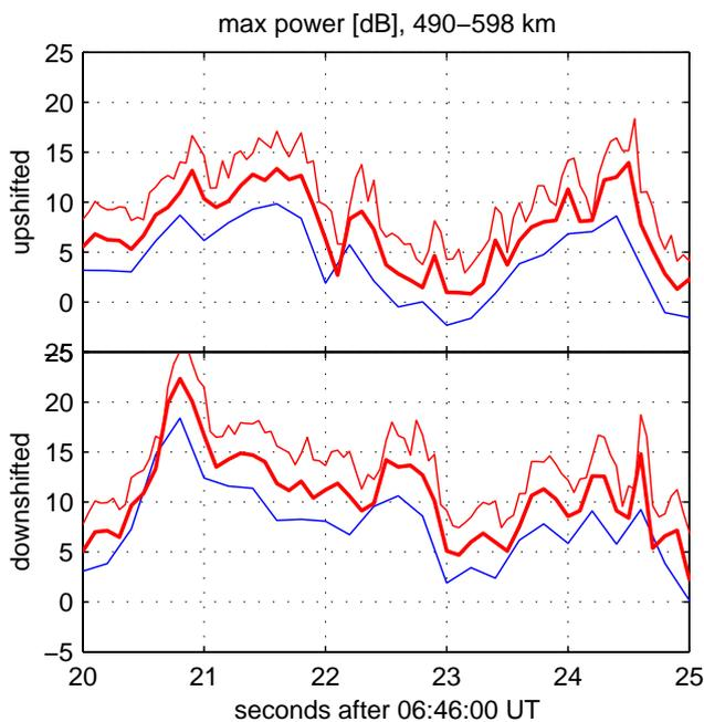
**Fig. 8.** Comparison of different integrations. The data is processed using three different integration periods: 50, 100 and 200 ms. Then, the maximum up- and down-shifted power per unit range and unit frequency within the range interval 490–598 km is extracted for each integration period, in order to obtain an idea of how the peak intensity varies with time. The 100 ms curve has been raised by 3 dB and the 50 ms curve by 6 dB, to keep them apart.
