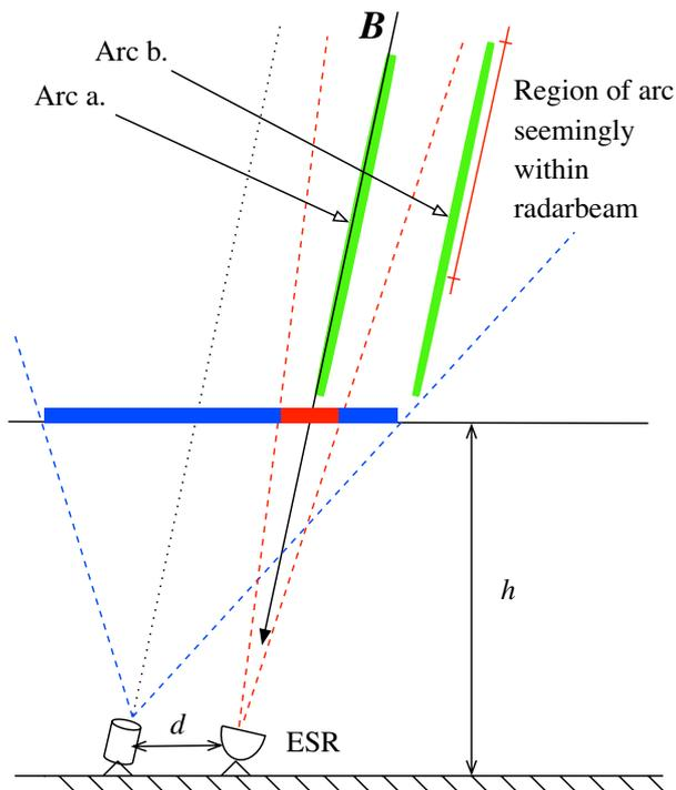
**Fig. 6.** Simple drawing depicting the experimental setup, highlighting the difficulties due to the distance between the two instruments. The camera (drawn as a cylinder) is located 7 km from the radar, almost directly north of it. Both the camera and the radar are pointing along the field.
