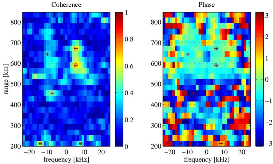
**Fig. 11.** An example of equal phase in both shoulders not captured by our technique, this is the 0.2 s integration starting at 06:46:15.60 UT. The two panels show coherence and phase, and the points investigated by the search algorithm are marked with a red circle when accepted, and with a red x, otherwise.
