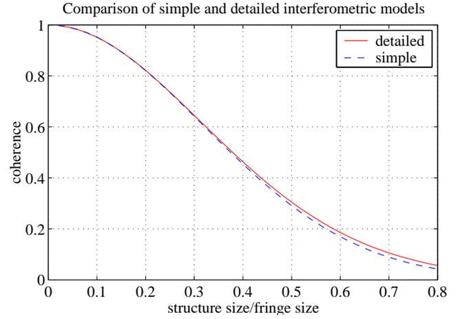
**Fig. 2.** Comparison of coherence computed using point antennas (dashed line) and Gaussian antennas, Eq. (12) (solid line), where the beam widths and separation of the EISCAT Svalbard Radar antennas have been used. The fringe size ( $= 1/2A$ ) corresponds to 234 m at 100 km range.
