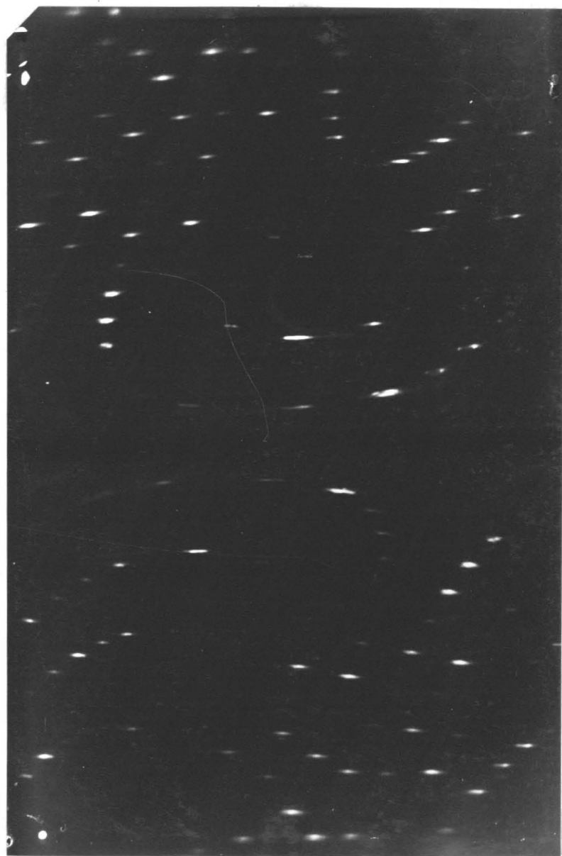
Fig. 3b First-layer Weissenberg photograph of \alpha - \text{In}_2\text{Se}_3 by the equi-inclination method
