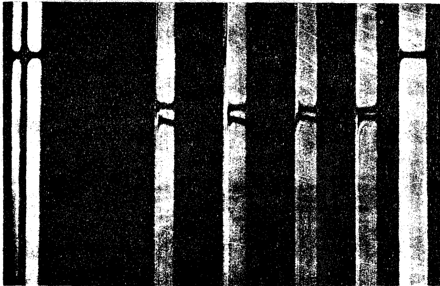
Fig. 5-5 A typical equilibrium pattern observed with schlieren optics.
