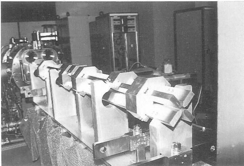
Photo. 4. RFQ electrode assembly on the way of getting put together using alignment jigs.
