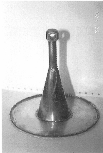
Photo. 2. The tapered inner conductor attached to the shorting plate.
