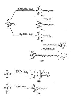
of benziltrimethylammonium hydroxide in chloroform to afford a practical light stabilizer 100.<sup>135)</sup> Besides, the reaction of 2,6-dimethylphenol with phthalic anhydride in the presence of  $ZnCl_2$ -catalyst at 130°C affording 101<sup>136)</sup> as well as the reaction of 1 with acetone and NaCN in N, N-dimethylformamide in a closed vessel at 140°C to afford 102<sup>137)</sup> are found in the literature.
