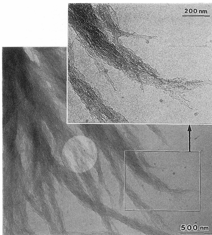
Fig. 3. Defocused image of PEEK solution-grown crystals. This image was taken at a few \mu\text{m} underfocus, and it reveals irregular-shaped microcrystals comprising a fibrillar lamella by defocus contrast 39 . The inset is a highly enlarged photograph of the corresponding rectangular area. Encircled is the area to give the electron diffraction pattern of Fig. 4. Fibrillar axis, namely the growth direction, corresponds to the b-axis.
