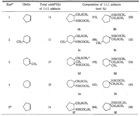
a) The isolation of the products formed by the ordinary two-component reactions was not put in practice. b) The yield represents pure compound isolated by column chromatography. c) A mixture of *cis*- and *trans*-isomers in an approximate ratio of 1: 6. d) One mol of ethyl cyanide was used instead of 1 mol of acetonitrile under otherwise identical conditions.
