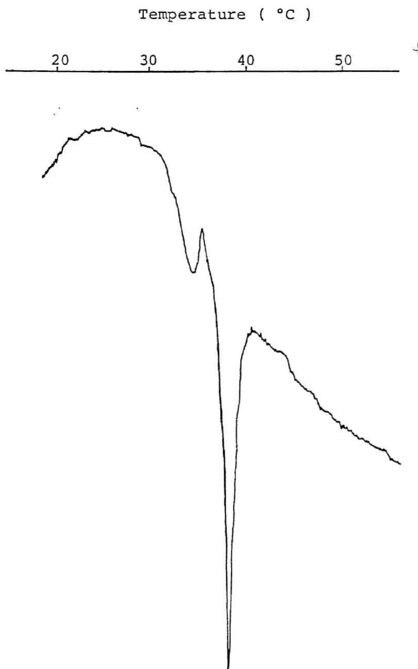
Fig.1 DSC curve of the flavoliposome. The flavoliposome was purified through centrifugation at 4 °C after sonication.
