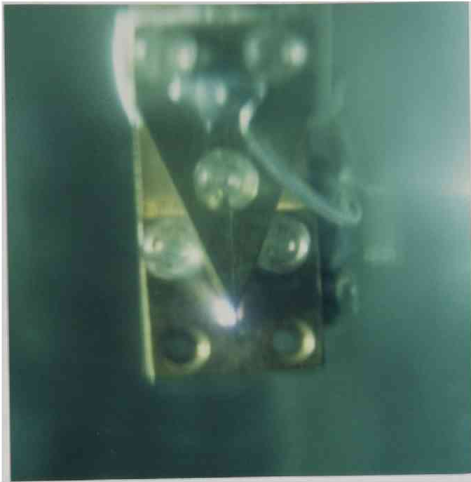
Figure 5.30: Photograph of QW-MIS LED at 77 K. Whitish purple emission was clearly observed.
