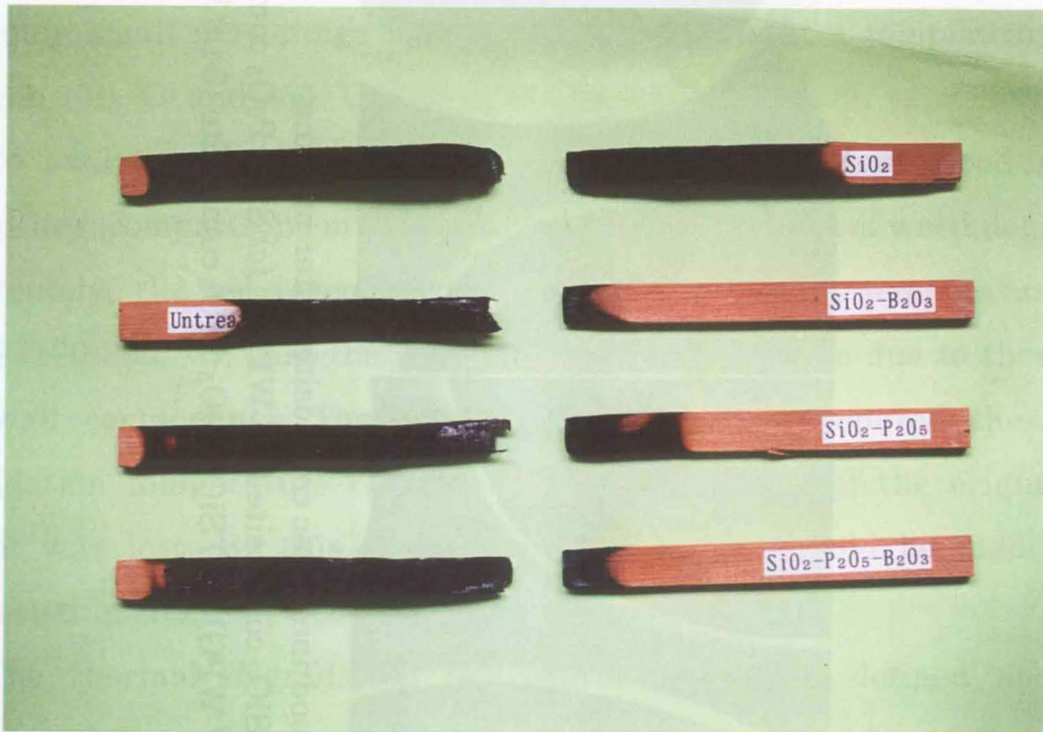
Fig. 3-13. Comparisons of the burned specimens after the fire-resistance test. Untreated plywood specimens (left) vs. various wood-inorganic composites (right).
