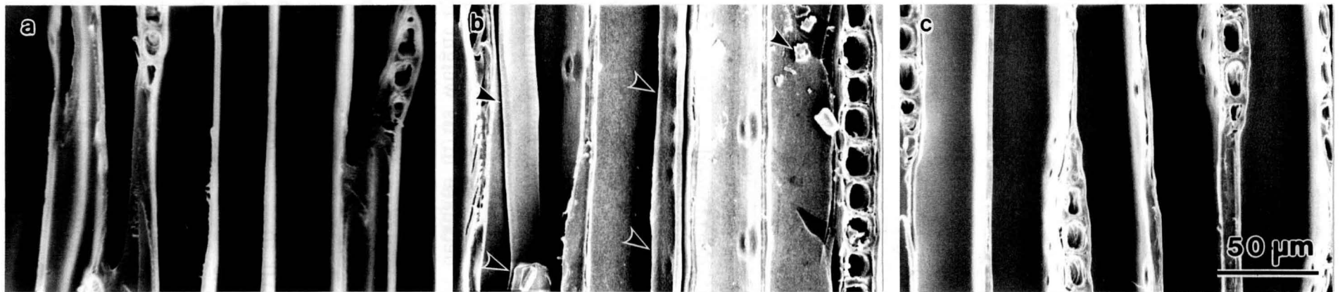
Fig. 6-1. Comparisons of SEM micrographs of untreated wood (a), Na 2 O-SiO 2 composites with SM (MTMOS/SM=0.03/0.03, 29.1 WPG) (b) and Na 2 O-SiO 2 composites with SA (MTMOS/SA=0.03/0.03, 21.2 WPG) (c).
