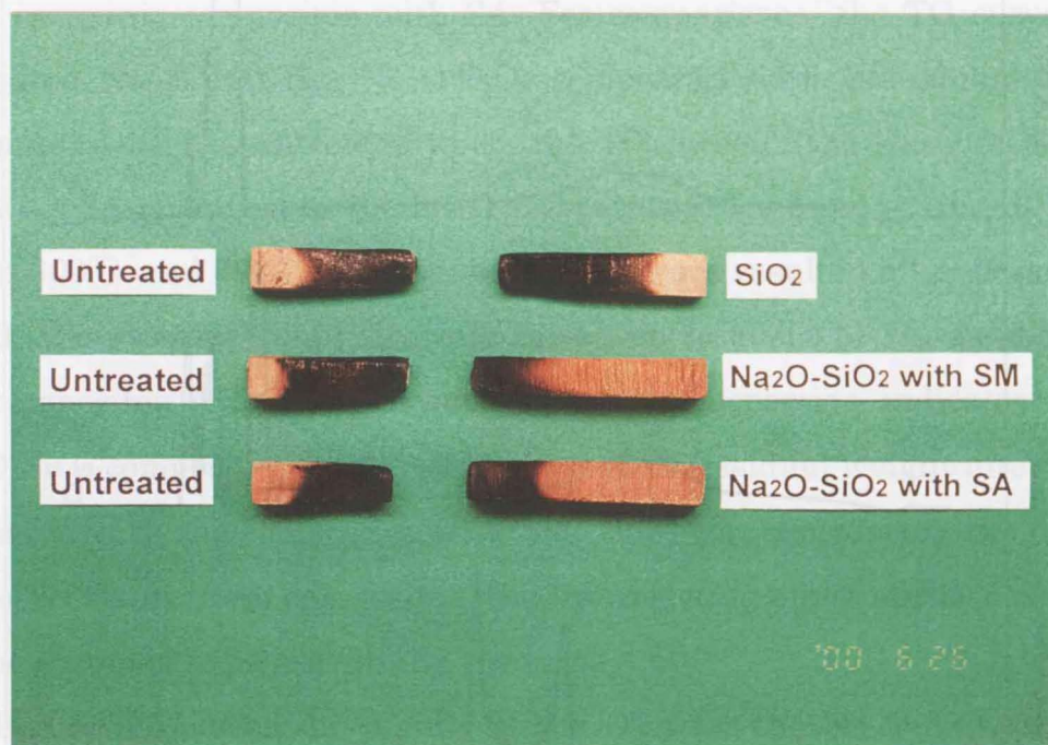
Fig. 6-6. Comparison of burned specimens after the fire-resisting test. Untreated wood specimens (left) vs. \text{SiO}_2 , \text{Na}_2\text{O}\text{-SiO}_2 wood-inorganic composites with SM and \text{Na}_2\text{O}\text{-SiO}_2 wood-inorganic composites with SA.
