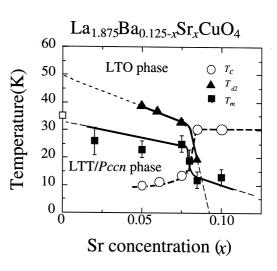
**Figure 1.** Phase diagram of LBSCO. Circles, triangles and squares denote the  $T_c$ , LTO-LTT(or *Pccn*) structural transition temperature  $T_{d2}$  by neutron scattering and the onset temperature for magnetic order  $T_m$  by  $\mu$ SR experiments, respectively.  $T_m$  for x=0 is quoted from [3]. Both solid and broken lines are guides to the eye.
