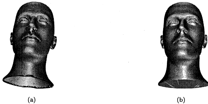
Figure 11: Reconstruction of the dataset MANNEQUIN (a) with boundary detection and (b) without boundary detection.
