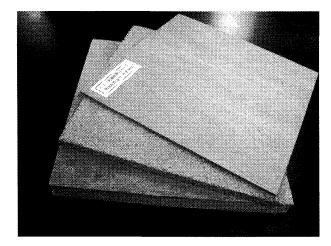
binderless boards was excellent while the board density were relatively low. The mechanical performance of binderless boards was improved with increasing the steam pressure and the longer pressing time contributed to the better dimensional stability. The chemical changes and self-bonding characterization of kenaf core is also investigated.
