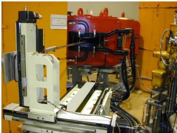
FIG. 10. (Color) Three-axes stage and model magnet aligned.
