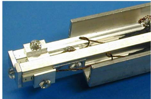
FIG. 11. (Color) Two Hall sensors MPT-141 installed on a two-axis holder. The axes of the Hall sensors intersect at right angles to each other.
