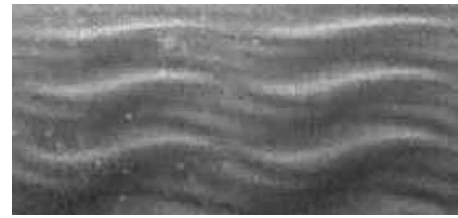
FIG. 4. The 3D flow obtained experimentally. R=100, \Omega=9.31 .
