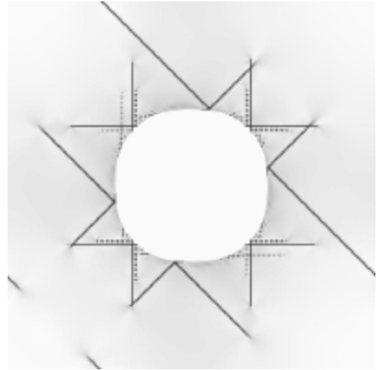
FIG. 6. Snapshot of e in Eq. (4.4) after dislocation formation, which is zero within the hard domain and nonvanishing outside. The slip lines end at dislocations.
