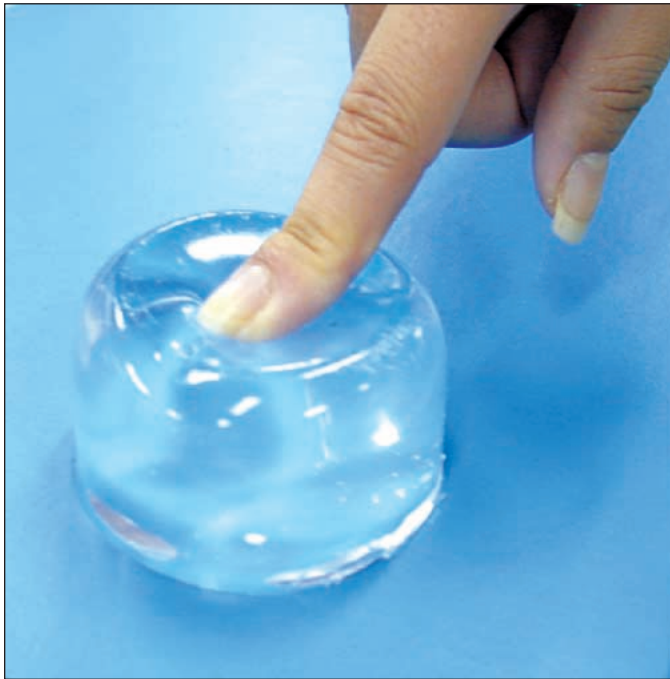
Fig. 11. Photograph of a homogeneous gel electrolyte. [Courtesy of Sanyo Electronic Co.]
