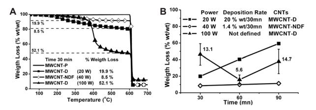
Figure 5. A) TGA of MWCNTs treated with plasma; B), TGA data for MWCNTs treated with plasma.
