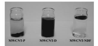
Figure 1. Dispersion in water tests of pristine nanotubes (MWCNT-P) and plasma treated nanotubes: MWCNT-D and MWCNT-NDF.
