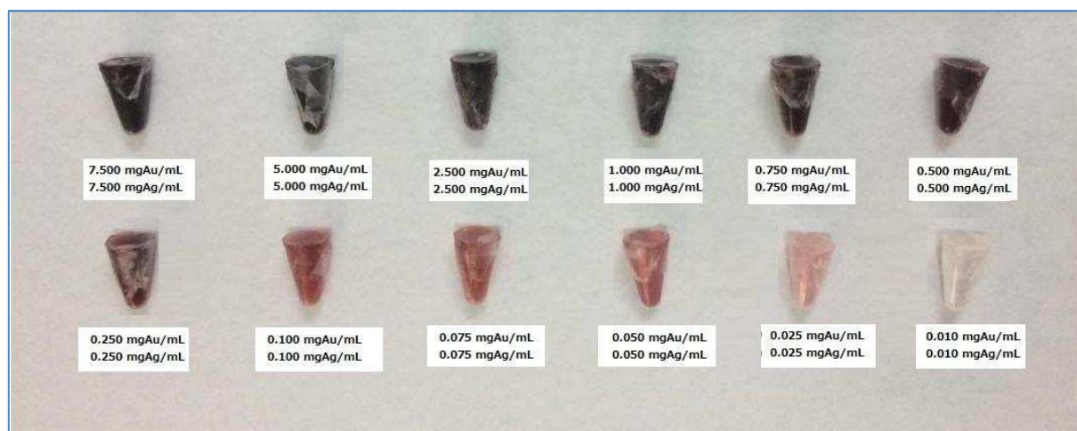
Fig. 2. Tumor phantoms with different GNPs and AgNPs concentrations ranging from 0.010 to 7.500 mg/mL.
